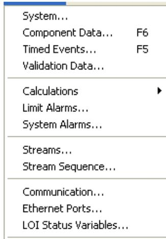
Many of the variables that a gas chromatograph uses during an analysis run—such as timed events, stream sequence, and calculation types—can be easily managed through MON 20/20.
