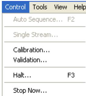
The options in the Control pull-down menu allow you to manage analysis runs as well as calibration, validation and baseline runs. Control menu commands also allow you to stop an analysis run immediately or at the end of the run.
