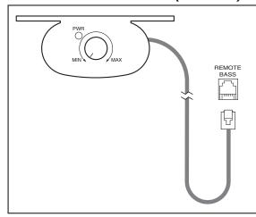
Remote level control allows the input level to be adjusted from an alternate location. It can be mounted under-dash or in-dash.
