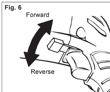
1. For **forward** (clockwise) rotation, push the forward/reverse lever to the left (when viewed from the back of the tool) as shown.
