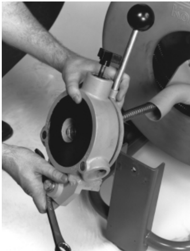
Figures 4a and 4b – Use 3/4" Wrench to Remove Powerfeed Assembly
