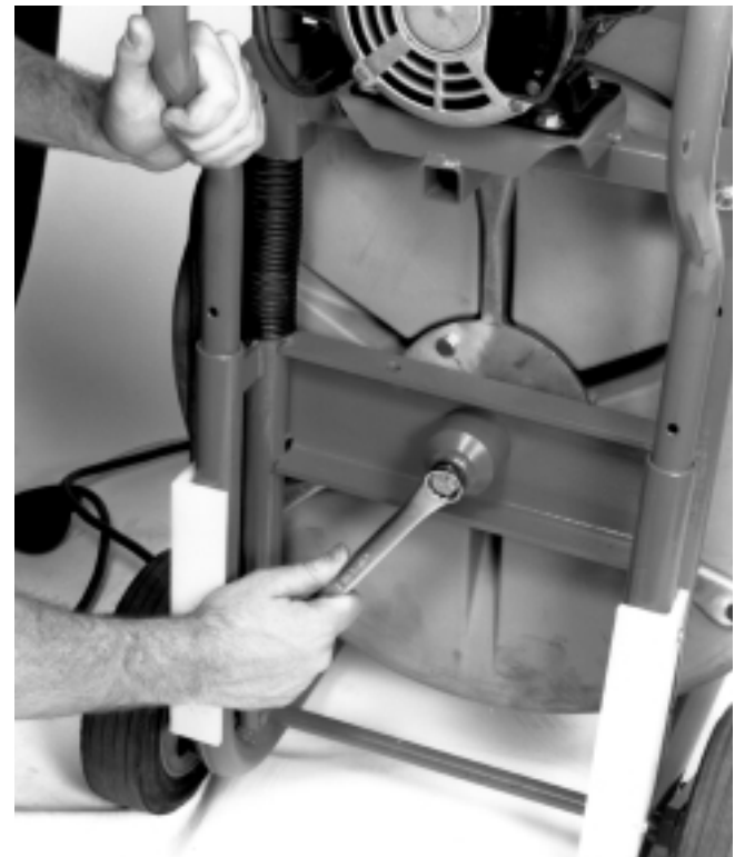
Figure 6 – Remove Bolt Which Fastens Drum Assembly to Machine Frame
