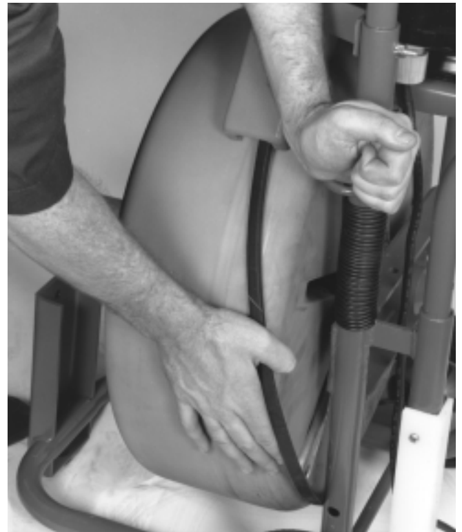
Figure 5 – Release Belt Tension
