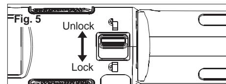
When the battery is installed, the tool is in operating condition. The lock switch prevents accidental starting by locking the forward/reverse switch. Always set the lock switch to "lock" before performing maintenance, changing accessories, storing the tool and any time the tool is not in use.
