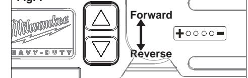
Press and hold the forward/reverse switch up for forward rotation, and down for reverse rotation. The switch will automatically return to the center, OFF position when it is released.
