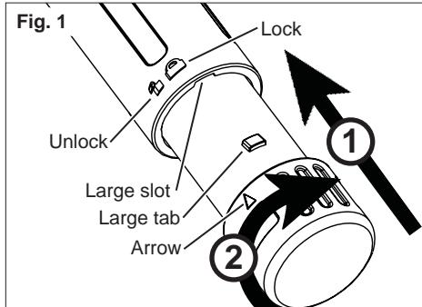
Line up the the large and small tabs on the battery with the large and small slots in the tool opening. Slide the battery all the way into the tool. Turn the battery clockwise to lock it in place. The arrow on the battery will line up with the
