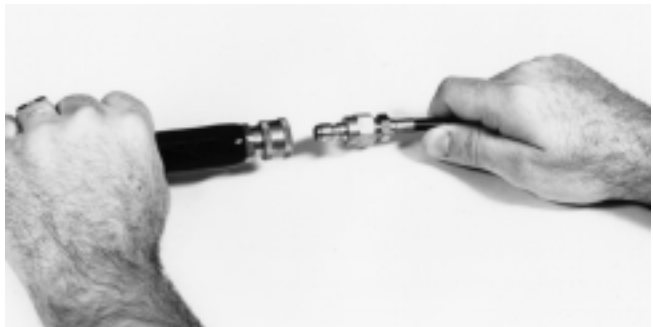
Figure 2 – Connect jetter hose to jetter
