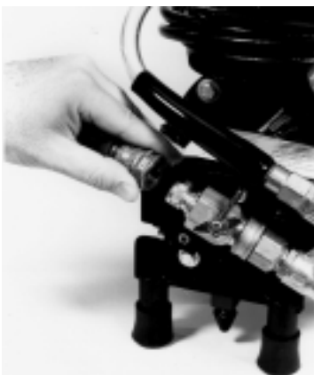
Figure 1 – Connect water supply hose to jetter. Close inlet supply valve (shown in closed position.)
