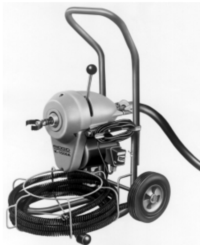
Figure 8 – Storing Cables on “A” Frame Models Only
