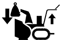
Weight Transfer Lift Handle To Engage
