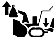
Weight Transfer Depress Pedal To Disengage
