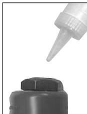
**⚠ WARNING** Any excess oil in the motor is immediately expelled from the exhaust port. Always direct exhaust port away from people or objects.
