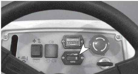
**2.** Check all switches, buttons, levers, pedals and steering to make sure they operate properly then turn key off.
