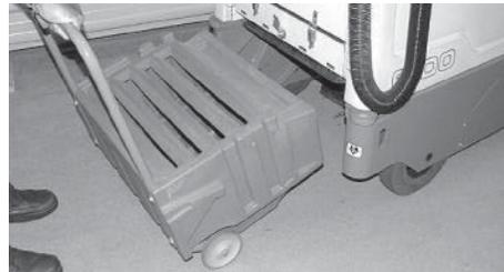
**4.** Make sure the hopper dust filter is properly installed and clean.
