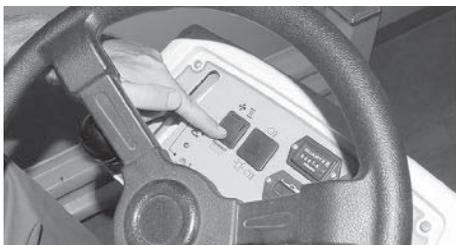
**2.** Turn key off, set parking brake and empty the debris hopper.
