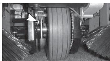
**5.** Check condition and tension of belts and chains. Lubricate the chains with SAE 30 Engine oil.
