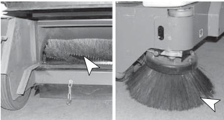
**6.** Check the brush skirts for damage, wear and adjustment. Replace if worn or damaged.
