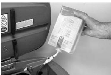
7. *FaST Model* - Check FaST-PAK supply hose for proper connection.
