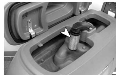
6. *FaST Model* - Check FaST-PAK level. Replace PAK as needed.
