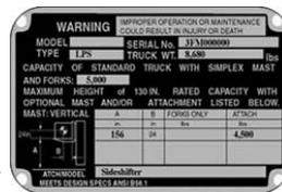
This data label indicates that this forklift has a 156" upright mast height in column A and a 24" load center in column B. Its stated capacity is 5,000 lbs with just its forks. With the side-shifter attachment, its stated capacity is 4,500 pounds.
