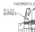
9. Push in control knob all the way and hold in. Immediately light the pilot with a match. Continue to hold the control knob in for about one (1) minute after the pilot is lit. Release knob and it will pop back up. Pilot should remain lit. If it goes out, repeat steps 5 through 9.
