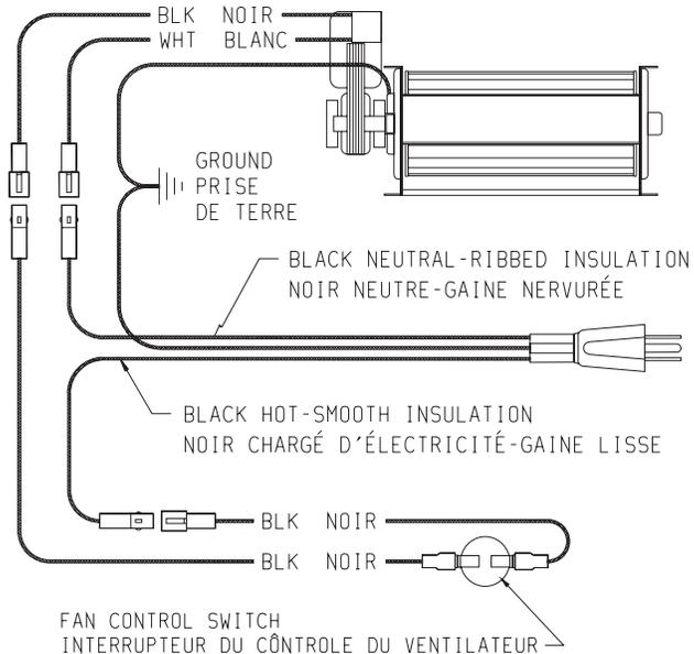
IF ANY OF THE ORIGINAL WIRE AS SUPPLIED WITH THIS UNIT MUST BE REPLACED, IT MUST BE REPLACED WITH 125°C WIRE OR ITS EQUIVALENT. S'IL Y A UN FIL ORIGINAL FOURNI AVEC L'APPAREIL QUI DOIT ÊTRE REMPLACÉ, IL DOIT ÊTRE REMPLACÉ AVEC UN FIL DU GENRE 125°C OU L'ÉQUIVALENT.
