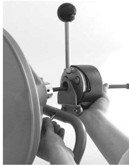
Figure 3 – Mounting Auto Feed Onto The Frame
