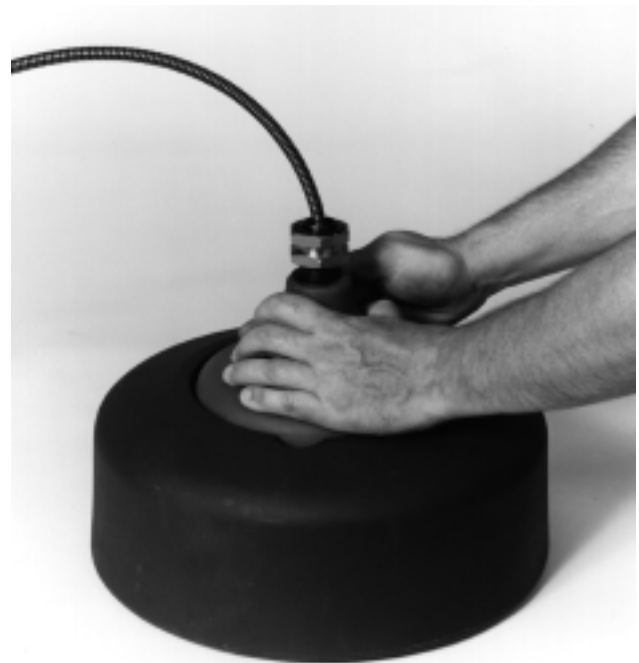
Figure 10 – Removing Cable End
