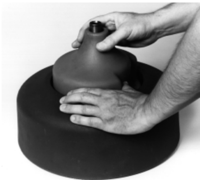
Figure 11A – Removing Inner Drum
