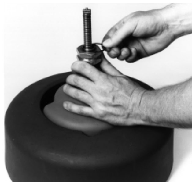
Figure 13 – Reassemble Inner Drum, Front Bracket and E-Rings
