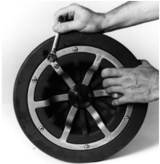
Figure 9 – Loosen Cable Bracket
