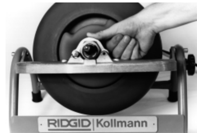
Figure 3 – Locking Front Bracket
