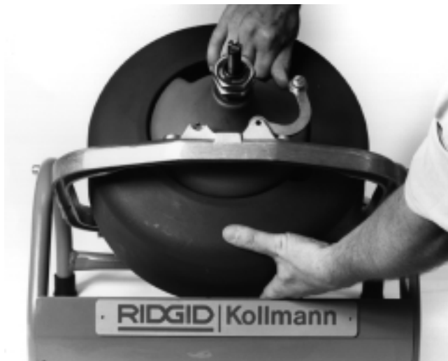
Figure 2 – Aligning Drum and Gearbox Bore
