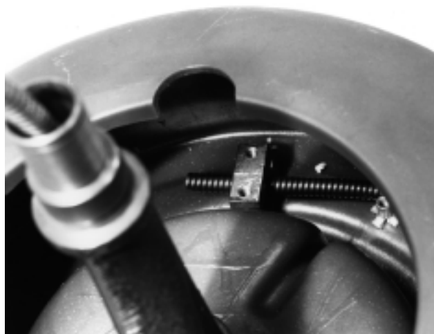
Figure 12 – Position New Cable Under Bracket
