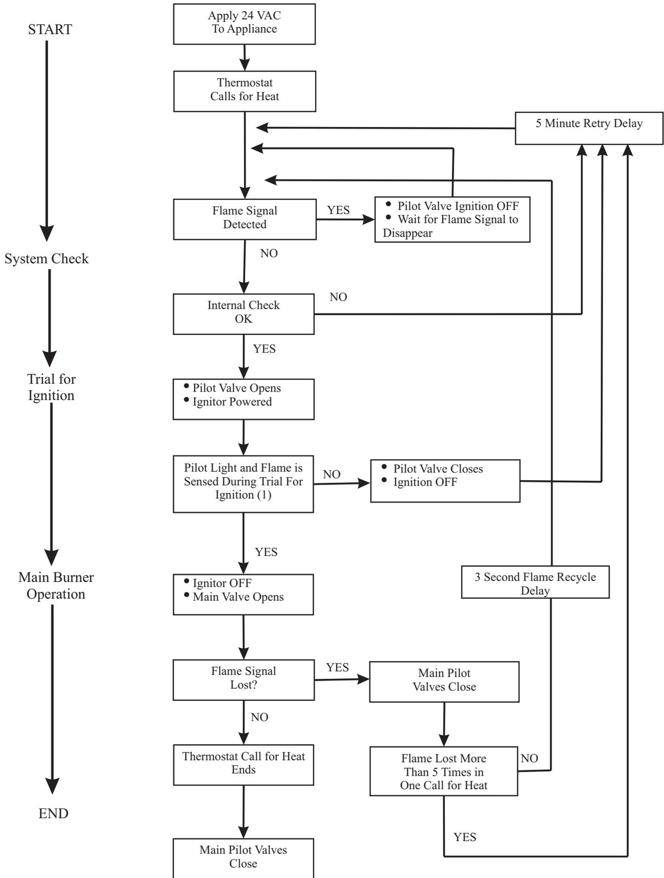
(1) Ignitor will turn OFF about 30 seconds into the trial for ignition if the pilot flame has not lit. It will turn back ON for the final 30 seconds of the 90 second trial for ignition. The pilot valve will be energized during the entire trial for ignition. This is normal operation for this gas ignition system.
