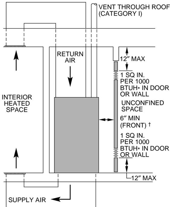
\* Minimum opening size is 100 sq. in. with minimum dimensions of 3 in.
