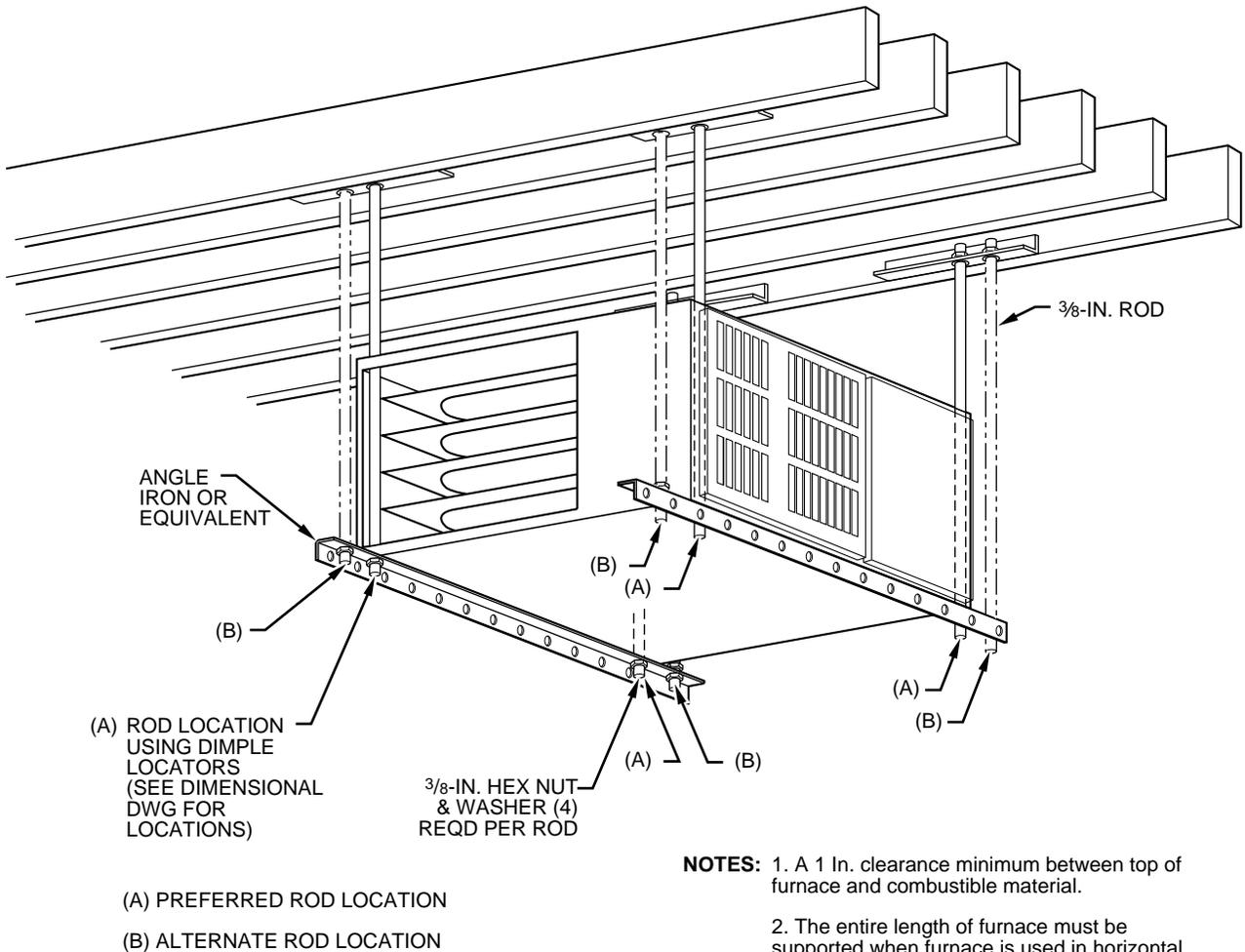
**Fig. 10—Horizontal Crawspace Installation on Hanger Rods**
