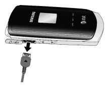
Remove the adapter from the phone by gently pulling the connector out and replace the plastic cover back over the open jack.
