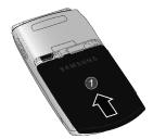
With the battery in position on the phone, place the cover back on the handset and slide it in until it clicks
