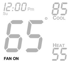
**Fan On** indicates constant fan operation. This feature is active even if the thermostat is set to **Off**.
