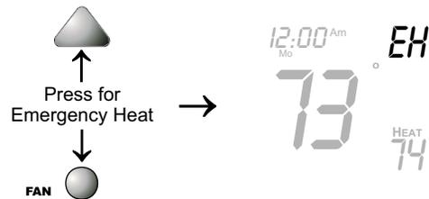
During Emergency Heat the thermostat will turn on the fan and the 2nd stage of heat, when there is a demand for heat, locking out the 1st stage compressor. Exiting Emergency Heat is the same as entering. During Emergency Heat only OFF and HEAT are available.
