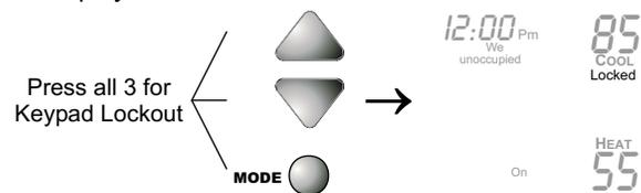
To **unlock** the buttons, again press and hold the Mode button. While holding the Mode button in, press the Up and Down buttons in together. The **Locked** icon will disappear from the display.
