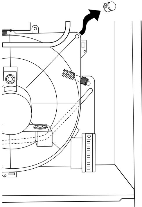
**Fig. 46—Inducer Housing Drain Tube**
