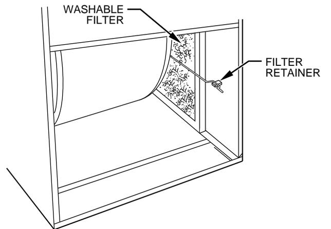
**Fig. 18—Filter Installed for Side Inlet**
