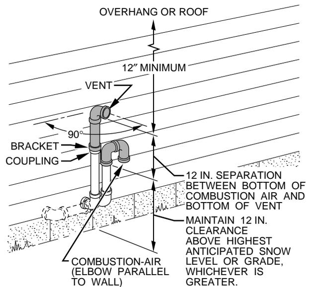
**Fig. 35—Sidewall Termination of Less than 12 in.**
