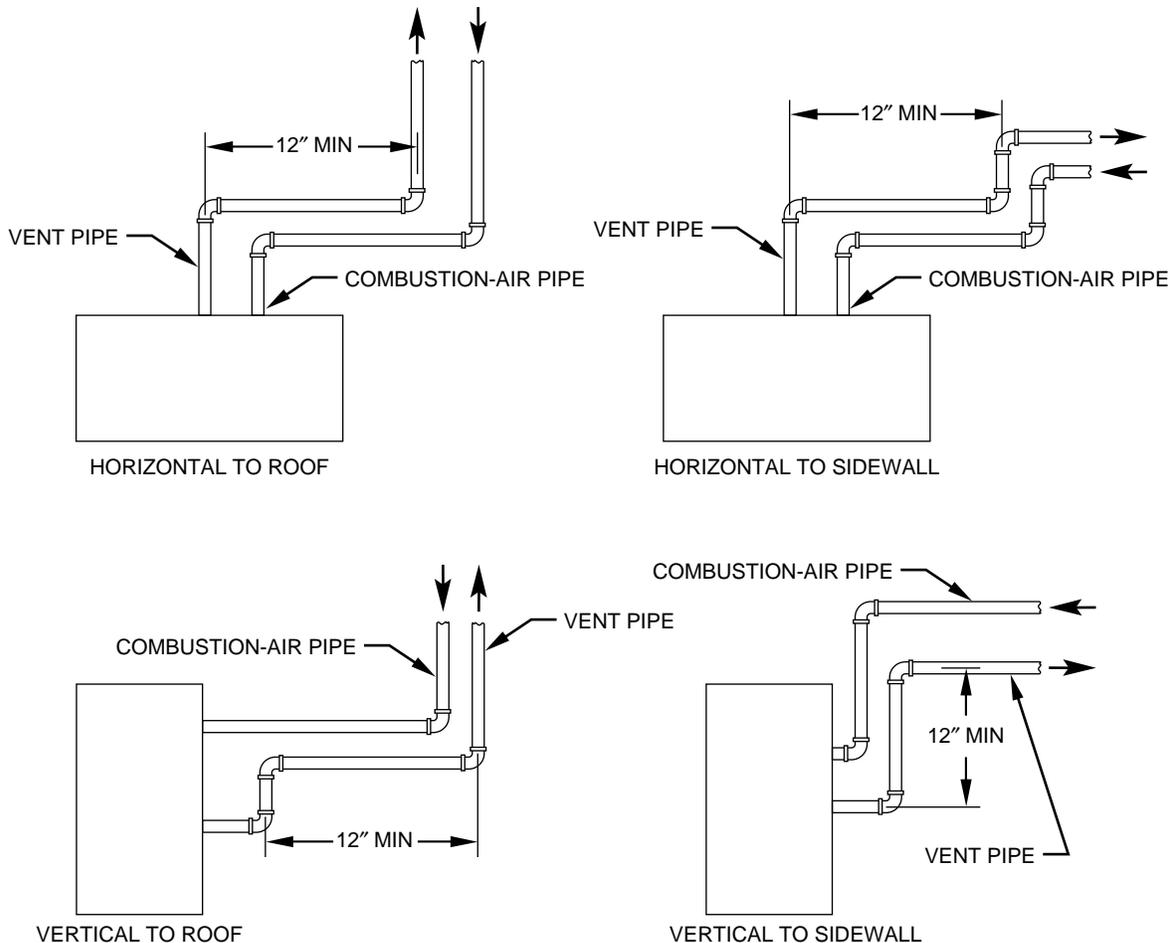
**NOTE:** A 12 in. minimum offset pipe section is recommended with short (5 to 8 ft) vent systems. This recommendation is to reduce excessive condensate droplets from exiting the vent pipe.
