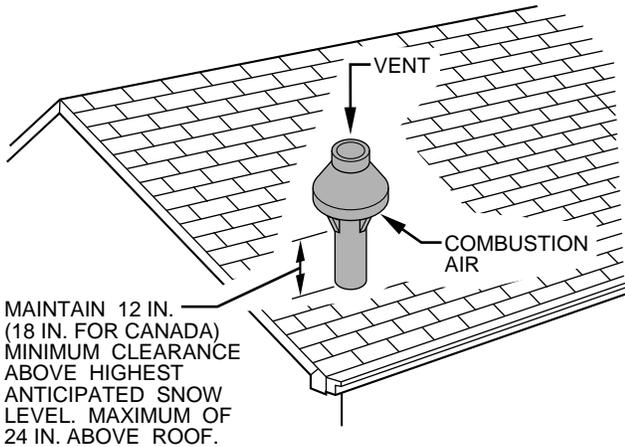
**Fig. 32—Concentric Vent and Combustion-Air Roof Termination (Preferred)**
