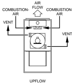
**NOTE:** Select 1 vent pipe connection and 1 combustion-air pipe connection.
