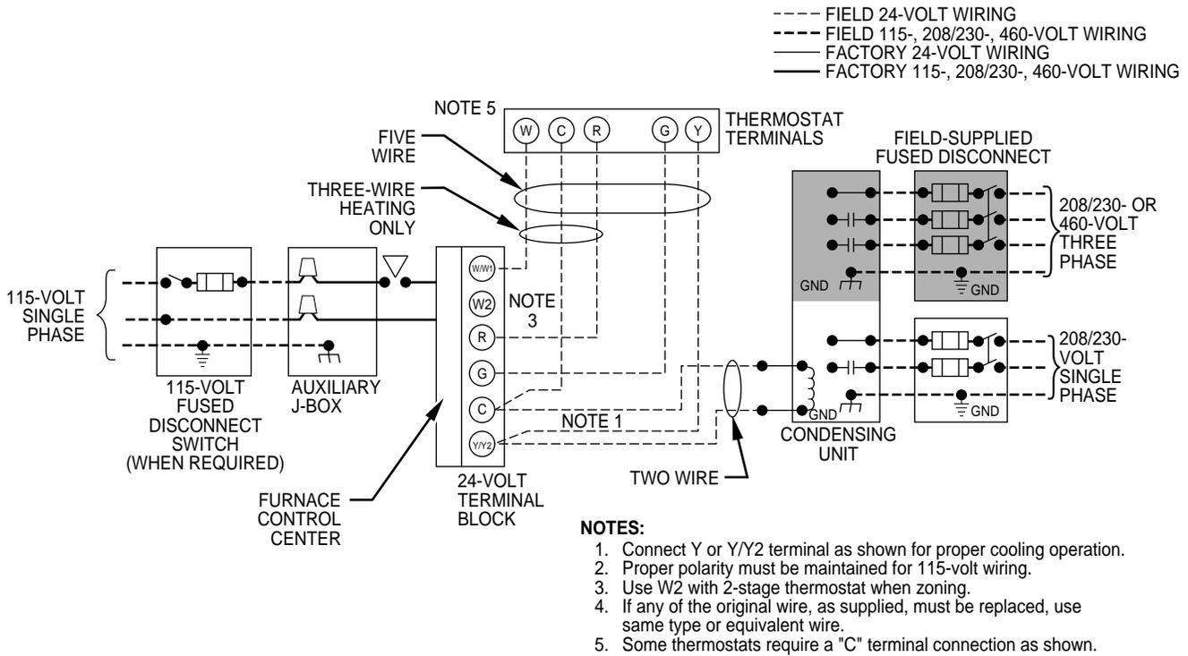
→ Fig. 22—Heating and Cooling Application Wiring Diagram
