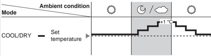
ECONAVI is activated, the unit maintains set temperature until a high sunlight intensity is detected. The sunlight sensor detects sunlight intensity during weather or day/night changes, and the unit adjusts temperature.
