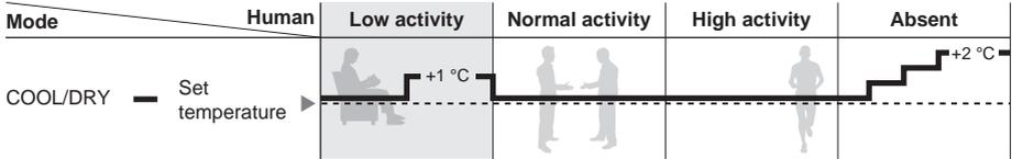
**AUTO COMFORT** ; Detecting human presence and activity, the unit controls room temperature to keep human comfortable consistently.
