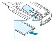
4. Place the battery so that the tabs on the end align with the slots at the bottom of the phone.
