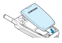
5. Press the battery until it clicks into place. Make sure that the battery is properly installed before switching the phone on.
