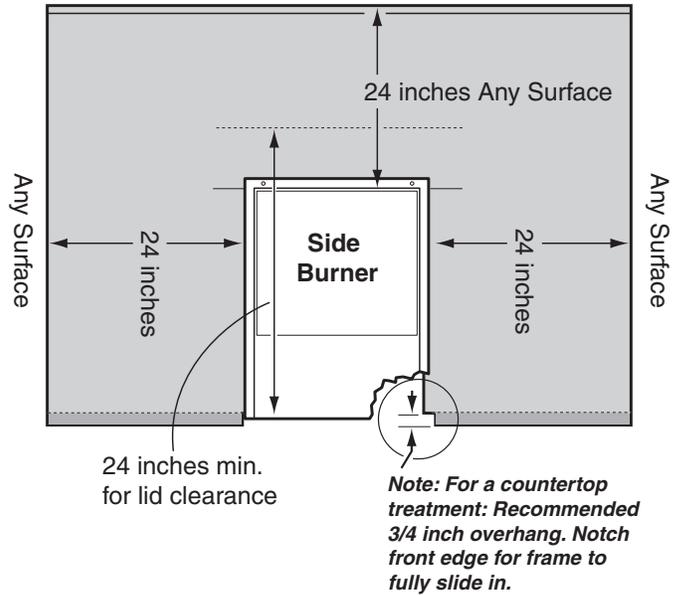
**⚠ WARNING:** All counter top finished surfaces must be constructed of a noncombustible material.
