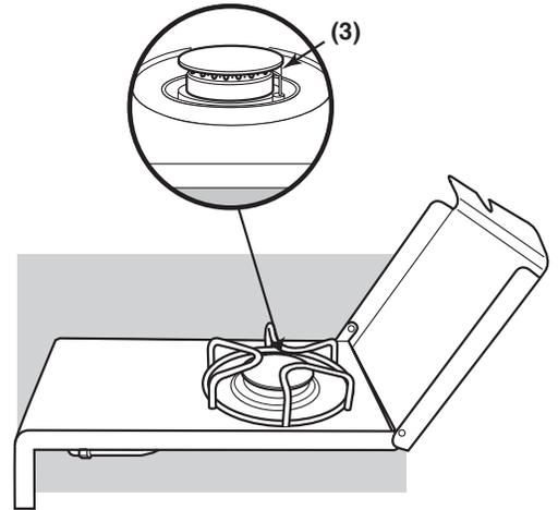
Make sure wire is connected between the igniter and electrode. Spark should be a white/blue color, not yellow.
