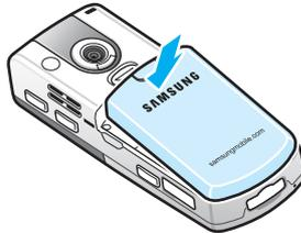
Make sure that the battery is securely locked before switching on the phone.
