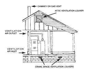
Application located in confined spaces. Ventilation air from inside building - combustion and draft hood dilution air from outside. Ventilated attic or ventilated craw space.
