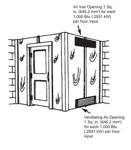
Illustration showing air opening necessary to supply air for combustion when heating appliance is installed in an enclosed room.
