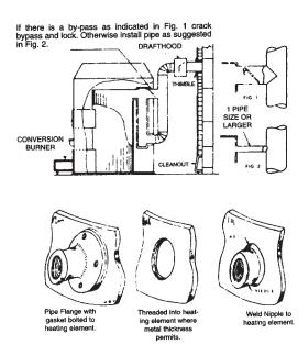
Suggested method for installing by-pass connection.
