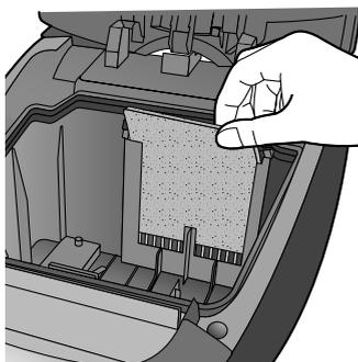
**D-14** Return the pre-motor filter to its original position.
