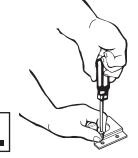
Line up holes in anti-tip bracket with mounting holes in floor. Use the screws provided to fasten anti-tip bracket to floor.
