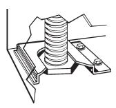
Carefully move range into final position. Look under range (a flashlight may be needed) to check that left rear leveling leg is engaged in the anti-tip bracket. If leveling leg is not properly engaged, remove and reposition the anti-tip bracket to ensure that the leveling leg fits
