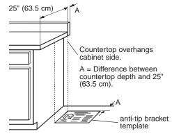
If countertop is not flush to the side of the cabinet opening, align the left side of the template to allow for the countertop overhang. Tape the freestanding range anti-tip bracket template in place.
