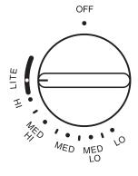
If burners do not light properly, turn cooktop control knob to the "OFF" position. Check that the power supply cord is plugged in and the circuit breaker or fuse has not blown. Check that the gas shutoff valves are set to the "OPEN" position. Repeat Step 22. If a burner does not light at this point, contact your KitchenAid dealer or authorized service company for assistance.
