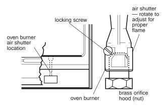
If the oven flame needs to be adjusted, locate the air shutter near the center rear of range. Loosen the locking screw and rotate the air shutter until the proper flame appears. Tighten locking screw.
