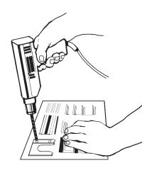
To mount anti-tip bracket to wood floor, use the anti-tip bracket template to mark where to drill mounting holes. Use a drill with a 1/8" (0.3 cm) drill bit to drill the two mounting holes. Remove template from floor.
