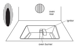
Check the oven burner for proper flame. This flame should have a 1/2" (1.3 cm) long inner cone of bluish-green, with an outer mantle of dark blue, and should be clean and soft in character. No yellow tips, blowing or lifting of flame should occur.
