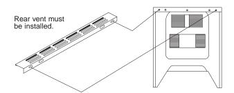
If you have a slide-in range, remove the outside screws from rear trim on range. Use screws to attach rear vent to range.
