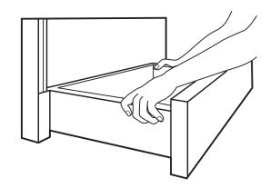
Insert storage drawer into slide rails on sides of drawer opening. Lift front of drawer slightly and push firmly to close drawer.
