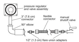
Assemble the flexible connector from the gas supply pipe to the pressure regulator, located in the lower left side
