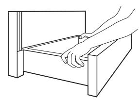
Press on front of storage drawer and release to open. Pull open to first stop position. Lift front of drawer to clear white wheels in drawer guides. Remove drawer and set it aside on a protected surface.
