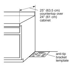
Place the anti-tip bracket template on the floor in the cabinet opening so that the left edge is against cabinet and the top edge is against the rear wall, molding or cabinet. If countertop is deeper than 25 inches (63.5 cm), measure and mark a distance 25 inches (63.5 cm) in from front of countertop opening and align template with mark (or subtract 25 inches (63.5 cm) from the countertop depth and add the difference to the corresponding dimension).
