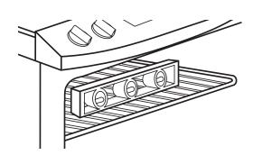
Place rack in oven. Place level on rack, first side to side; then front to back. If the range is not level, pull range forward until the rear leveling leg is removed from the anti-tip bracket. Adjust the leveling legs up or down. Then slide range back into position. Check that leveling leg is engaged in anti-tip bracket.
