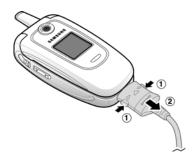
**Note:** Always unplug the adapter before removing the battery from the phone during charging; otherwise, the phone could be damaged.
