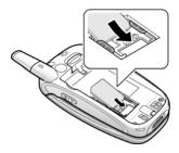
When you need to remove the SIM card, slide it upwards, as shown, and take it out of the socket.
