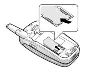
4. Replace the battery so that the tabs on the end align with the slots at the bottom of the phone.
