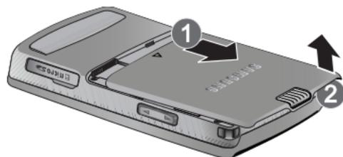
2. Lift the battery up (1) and away (2) from the phone, as shown.
