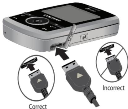
**Note:** The previous illustration is the correct and incorrect method for connecting the charger. If the incorrect method is attempted, damage to the accessory port will occur therefore voiding the phone's warranty.
