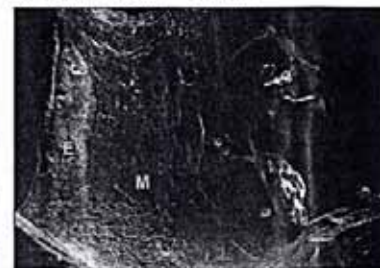
Fig 10: SEM microphotograph of an anorganic preparation of the medullary zone of a 50% \beta -TCP/50% HA specimen implanted for 4 months. The bone calcified matrix (M) is coating the ceramic (E). Bar = 100 \mu m.
