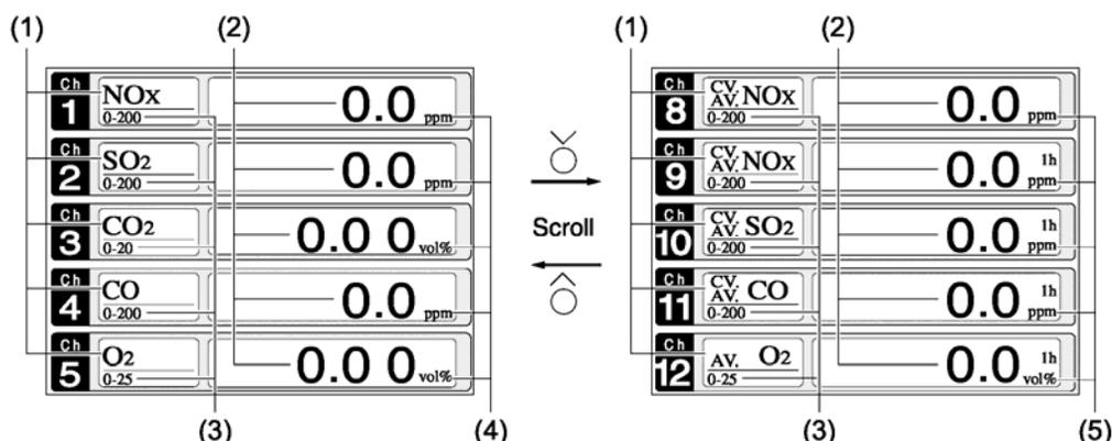
Scroll the UP and DOWN keys to display more than 5 channels.
