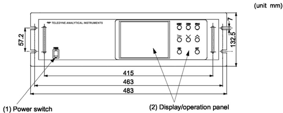
Figure 2-1A: Model 7500ZA Front Panel
