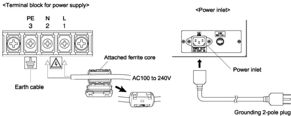
**CAUTION:** AFTER WIRING IS COMPLETE, BE SURE TO REPLACE THE PROTECTIVE COVER OVER THE TERMINAL BLOCKS.
