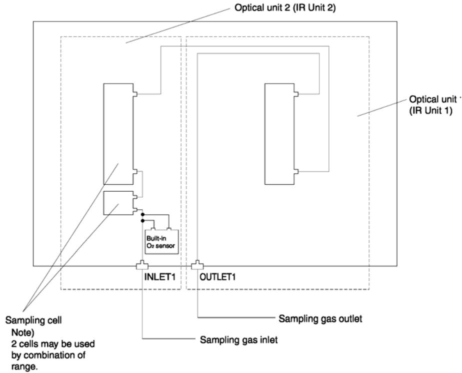
Correspondence between measured components and the optical units is as follows:
