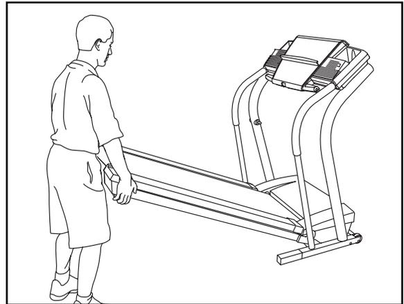
2. Move your right hand to the position shown and hold the treadmill firmly. Using your left hand, pull the latch knob to the left and hold it. Raise the treadmill until the latch pin is aligned with the indicated hole in the side of the treadmill. Insert the latch pin into the hole. **Make sure that the latch pin is fully inserted into the hole.**
