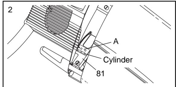
3. Connect the included short jumper wire (B) to the wire on the receiver (A). Connect the other end of the short jumper wire to the PLS2 jack on the underside of the Console (82). (Note: If there is already a wire in the PLS2 jack, unplug it.) Discard the other wires included with the receiver. Use the included wire tie to secure the wires, if needed.
