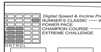
For about six seconds after a program is selected, the Incline/Distance display will flash the maximum incline setting for the program, and the Speed display will flash the maximum speed setting for the program. The Time/Pace display will show how long the program will last. The program display will show the first five speed settings of the program.
