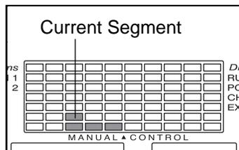
setting and an incline setting for the first segment, simply adjust the speed and incline of the treadmill as desired by pressing the Speed and Incline buttons. Every few times a Speed button is pressed, an additional indicator will light or darken in the Current Segment column.
