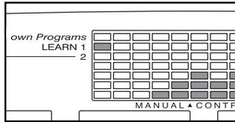
For about six seconds after a program is selected, the Incline/Distance display will flash the maximum incline setting for the program, and the Speed display will flash the maximum speed setting for the program. The Time/Pace display will show how long the program will last. **Note: If only three columns of indicators are lit in the program display, see HOW TO CREATE A CUSTOM PROGRAM on page 15.**
