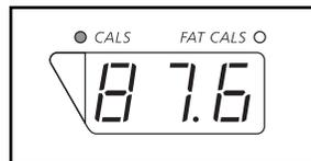
**Speed/Minutes-Mile display**—This display shows the speed of the walking belt and your current pace (pace is measured in minutes per mile). The display will alternate between one number and the other every seven seconds. Each time the Speed buttons are pressed, the display will show the speed setting.
