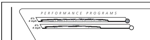
The profiles on the console show how the speed and incline of the treadmill will change during the performance programs. The numbers at the left ends of the profiles show the maximum speed and incline settings for the programs. For example, the upper left profile shows that the treadmill will reach a maximum incline of 6% and a maximum speed of 4 mph during the first program.
