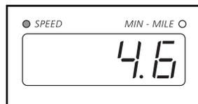
Note: The speed can be displayed in either miles per hour (mph) or kilometers per hour (kph). To see which unit of measurement is selected, first hold down the Stop button while inserting the key
