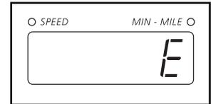
**Distance/Incline/Laps display**—This display shows the distance you have walked and the number of 1/4-mile laps you have completed. The display will alternate between one number and the other every seven seconds. Each time the Incline buttons are pressed, this display will show the incline setting.
