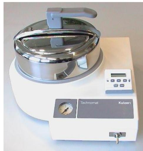
The functional design of the unit makes it simple and problem-free to operate. When the valve lever is moved upwards, the pressure is built up to a level of 2.0 bar. The pressure gauge within the unit housing indicates the operating pressure. The pressure is released by moving the valve lever downwards. The Technomat is a space-saving, compact unit. The housing is made from macrolon resin and the pressure pot itself is of INOX steel.
