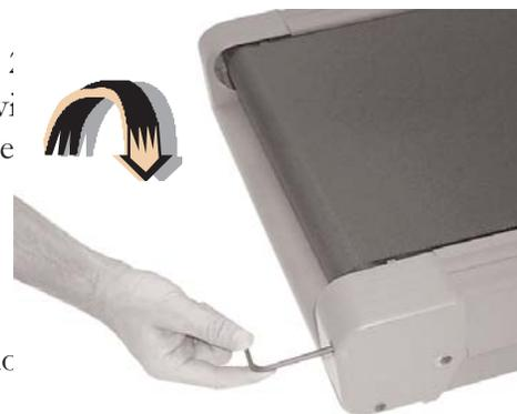
**WALKING BELT IS SLIPPING DURING USE** (Diagram 3)
