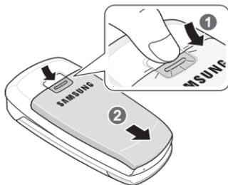
2. Carefully lift the battery cover away from the bottom of the phone.
