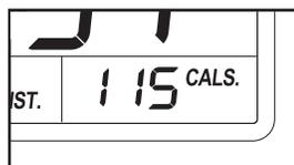
**The upper display**—The upper display can show the elapsed time, the distance that you have walked or run, the approximate number of calories that you have burned, or the speed of the walking belt. Press the Display button repeatedly until the upper display shows the information that you are most interested in viewing. Note: While information is shown in the upper display, the same information will not be shown in the lower left or lower right display.
