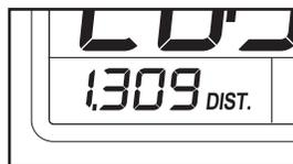
**The lower right display**—The lower right display can show the approximate number of calories that you have burned and the speed of the walking belt.
