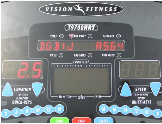
1. Press & Hold both “ELEVATION UP” and “SPEED DOWN” at the same time for 3-5 sec. Then, the dot vision display will show “DGB1J A564” and right display is show “ VERSION ”
