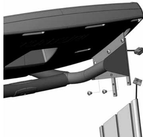
Turn the sliders located at the sides of the handlebars downward so that you can attach them with another screw (**F**) through the lower hole of the handlebar.
