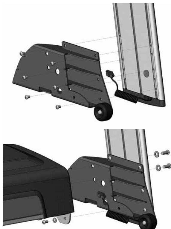
Secure the handrail mounting pieces to the lower ends of the handrails, using six hex screws (**A**) on each mounting piece. Tighten these screws carefully. **NOTE!** The left handrail and mounting piece are marked with a round red sticker. Secure both handrails to the running base with two hex screws (**B**) and washers (**C**) and with one hex screw (**D**) and a washer (**E**). Be careful not to
