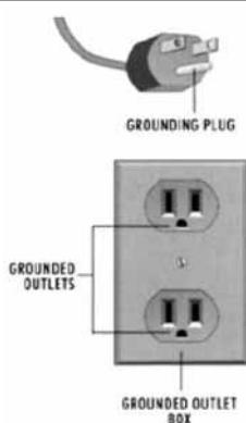
**DANGER!** Improper connection of the equipment-grounding conductor can result in a risk of electric shock. Check with a qualified electrician or serviceman, if you are in doubt as to whether the product is properly grounded. Do not modify the plug provided with the product - if it will not fit the outlet, have a proper outlet installed by a qualified electrician.
