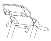
Connect the wire. After connecting the wire thread it into the handlebar then push the monitor onto the handrails. You may have to shake the handrails from side to side to get the monitor to fit. Once you have the monitor in place, secure and tighten the bolts on the monitor. Tighten all bolts. Remove the protective film from the display.
