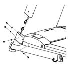
Connect the wires before you assemble the handrails. Secure each handrail with four washers and bolts. **NOTE:** Do not tighten these bolts until the horizontal handlebar and monitor have been secured.
