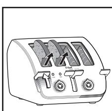
Toasting chamber automatically lifts toast and lever once toasting cycle is complete.
