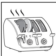
Toasting chamber automatically lifts bagel and lever once toasting cycle is complete.
