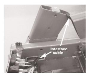
**Step 4:** Tilt the pedestal up and slide it down the pedestal supports, being careful not to pull out the upper wiring harness. Plug the upper wiring harness into the motor controller. Install the four 5mm x 15mm screws into the pedestal legs.
