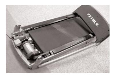
Detach the rubber band from the upper wiring harness and route the cable down the pedestal leg support and out the bottom hole as shown.
