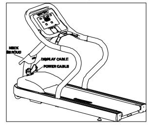
Slide the neck shroud up to gain access to the display cable. Connect the display cable to the base assembly power cord.
