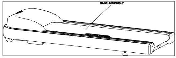
Remove all packaging material so the base assembly is sitting on the shipping crate platform. With a helper, lift the base assembly from the shipping crate platform, and place it in the location where it will be used. Be sure the selected location is level, and close to a power outlet.
