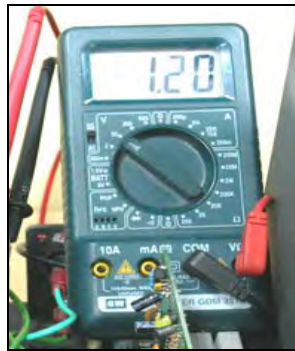
Step 3. Turn the VR gear until the multimeter shows 1.20 VDC.
