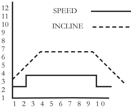
The Plateau Program is designed to gradually increase treadmill Speed and elevation in the first segment (warm up), and gradually decrease speed and elevation in the last segment (cool down).
