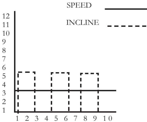
The Rolling Hills Program is designed to vary treadmill elevation while maintaining a constant walking belt speed.
