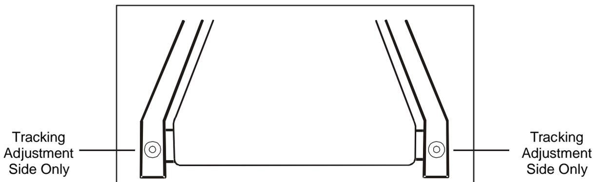
**Note:** Adjustment is thru small hole of end cap.
