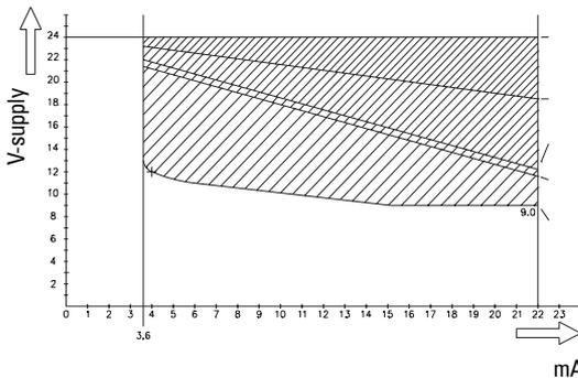
voltage drop over 250 ohm measuring resistance
