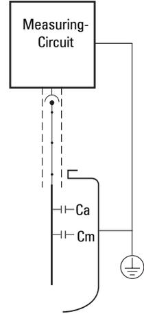
The measurement is further protected from interference by a buffer, which applies the frequency signal from the measurement section to the active shield section. This effectively eliminates any electrical potential difference between the shield and the measurement section and prevents additional changes in capacitance occurring.
