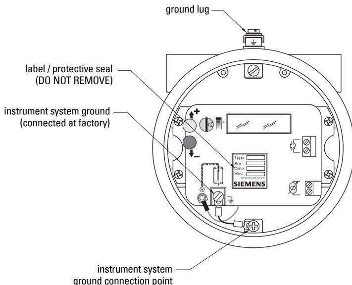
**! WARNING: When connecting the probe, do not leave moisture or metal scrap (from the cable shielding, for example) inside the housing. This could interfere with transmitter operation, or cause a short circuit.**
