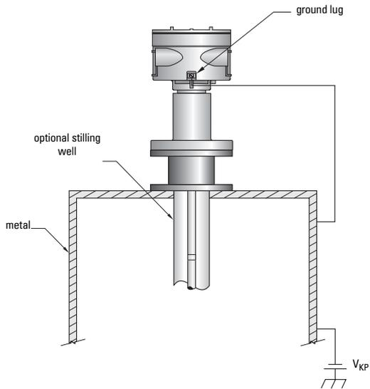
**Note:** Grounding the SITRANS LC 500 as illustrated above provides only system grounding for referencing purposes: it does not provide safety grounding.
