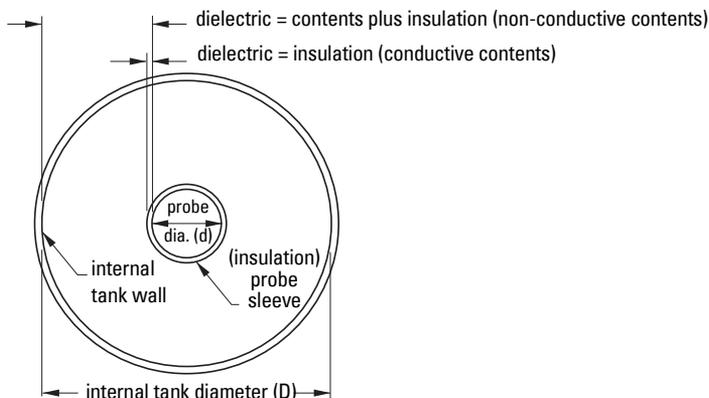
**Note:** For simplicity, the probe is shown centrally mounted. If it is to be mounted off-centre, take care to ensure the electrode remains parallel to the tank wall.
