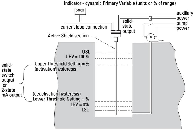
3. Upper Threshold Setting and Lower Threshold Setting activate and deactivate the 2-state output, and/or the solid-state output: the settings can be modified to adjust the hysteresis (the window within which the probe is considered 'covered').
