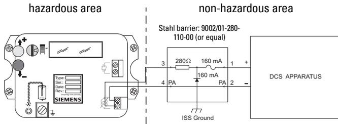
When Ex applications are using an Ex approved Intrinsically Safe (I.S.) power supply unit, no barrier is required and grounding is optional.
