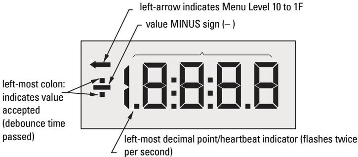
The LCD will hold information for a long time even when not refreshed (for example, if there is a loss of power). The heartbeat indicator blinks continuously whenever the device is working. A still heartbeat signals that the device has stopped working.
