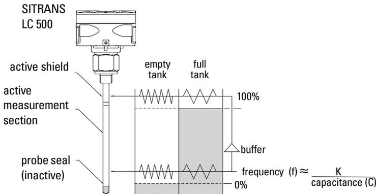
The relative lengths of the measurement section and active shield section can be specified to suit a particular application. If the measured range will be short relative to the total length of the electrode, specify a short measurement section. This increases the achievable resolution of the measurement, since any change in level will be greater relative to the length of the measurement section.
