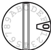
The rotary switch has a small slot where the current position can be read. The positions are read clockwise, and in increasing order: 0, 1, 2, 3, 4, 5, 6, 7, 8, 9, A, B, C, D, E, and F. The position wraps from F to 0.
