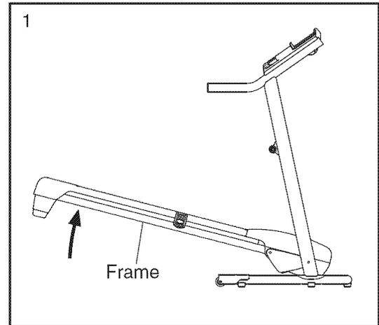
2. Move your right hand to the position shown and hold the treadmill firmly. Using your left hand, pull the latch knob to the left and hold it. Raise the frame until the catch is past the latch pin, and then slowly release the latch knob. **Make sure that the frame is held securely by the latch pin.**
