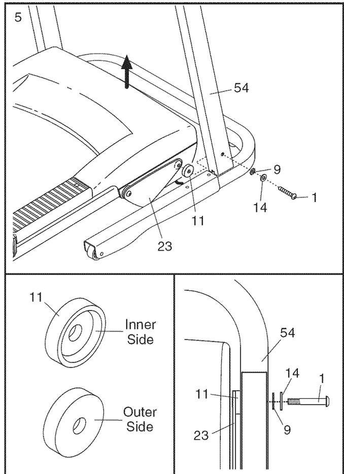
6. **See the left inset drawing.** Identify the outer side of the remaining Frame Spacer (11).
