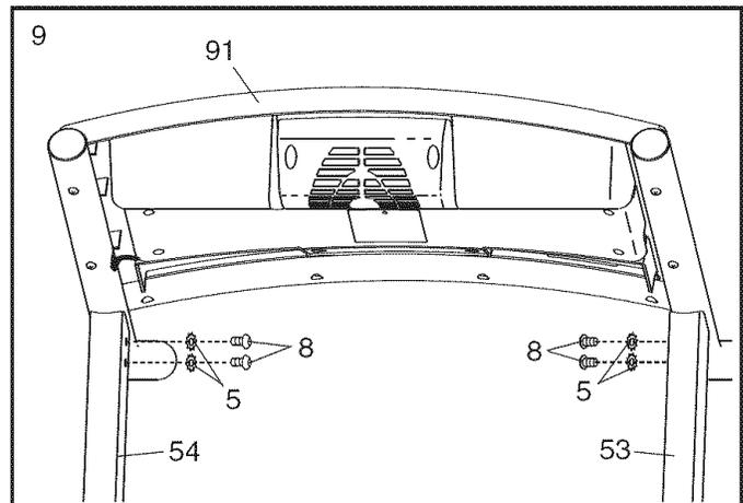
10. Start two M8 x 15mm Bolts (8) with two M8 Star Washers (5) into the Uprights (53, 54). **Then, firmly tighten all six M8 x 15mm Bolts (see step 9).**
