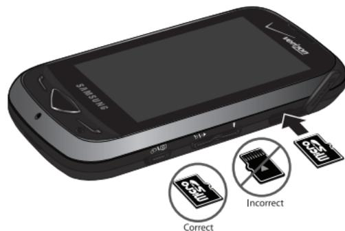
2. Push the microSD card into the slot until it locks into place.
