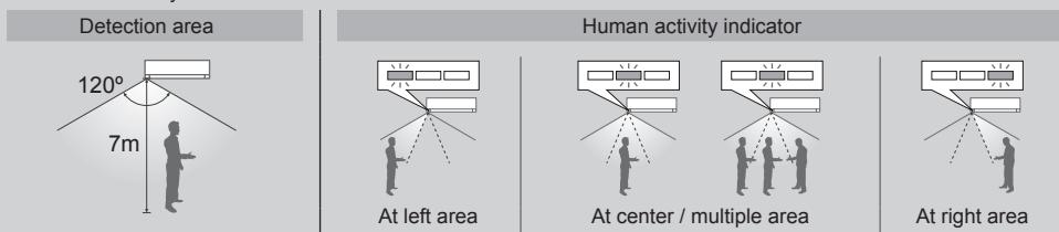
The unit judges human activity area for a few seconds before indicator updates. Based on area activeness horizontal airflow direction louver will adjust either fix at predetermined position or swing left/right periodically.
