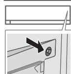
Use when remote control is misplaced or a malfunction occurs. Raise the front panel:
