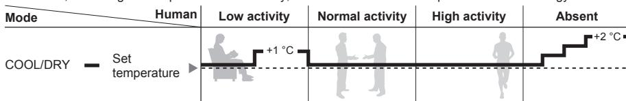
**AUTO COMFORT** ; Detecting human presence and activity, the unit controls room temperature to keep human comfortable consistently.
